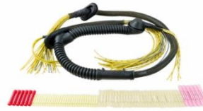
Item Number: 2016046-2TN Model: E46 Touring / Caravan Repair set wire harness Year of construction: 10.99 - 02.05 Installation: Rear hatch right Preassembled: Butt connector, Heat shrink connector Numbered wires
